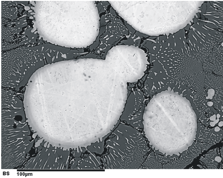
Figure 1. EPMA backscattered electron image of iron alloy blebs of SM (white) in quenched LM. Darker rims on the blebs crystallized during quenching. Experiment at 1200 °C with minor abundances of W and Si.
